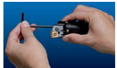
3. Tighten three screws to clamp the boring head. Use short screws for upper clamping hole and long screw for bottom clamping hole.
